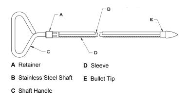
Dimensions of the LivaNova Tunneler were optimized to minimize risk of damage to Lead connector(s) that may occur with the use of general-purpose tunnelers.
